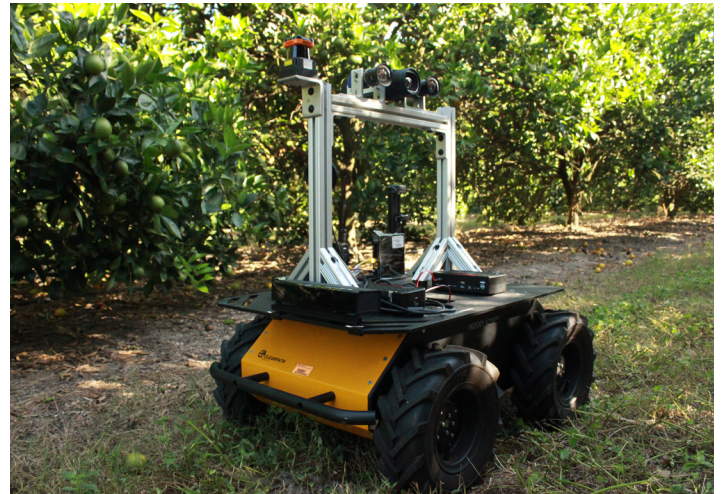
(LEFT) Dr. Wonsuk “Daniel” Lee (left) and ABE alumnus Hao Gan (right) uses an autonomous robot for immature green citrus fruit yield mapping and imaging design platforms for automatic strawberry counting. (RIGHT) This citrus yield mapping robot is used by Dr. Wonsuk “Daniel” Lee and ABE alumnus Hao Gan to count the number of fruits on citrus trees and can create a yield map of the citrus grove.
