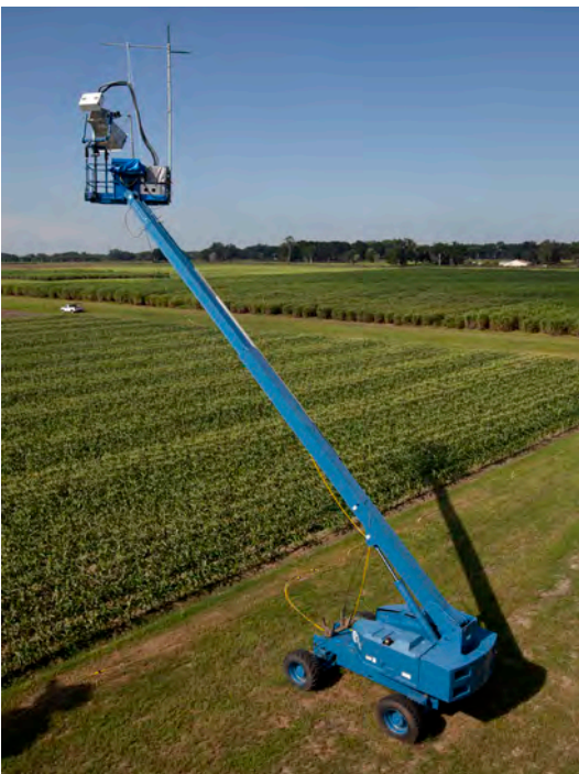
The UF-L-band Automated Radar System observing microwave signatures during a growing season of corn.
