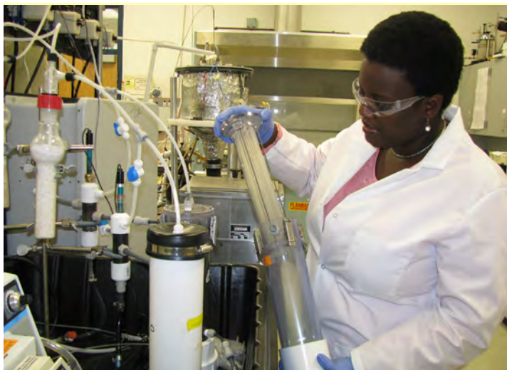
Graduate student Stephanie Burrs examines the Hollow Fiber Membrane Bioreactor (empty reactor with fibers shown) which is expected to improve performance of anaerobic digestion (AD). Preliminary results show reductions in hydraulic retention rate (HRT).
