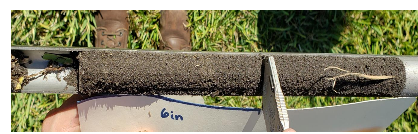
Figure 3. Cutting soil sample to depth of 15 cm (6 in.)
