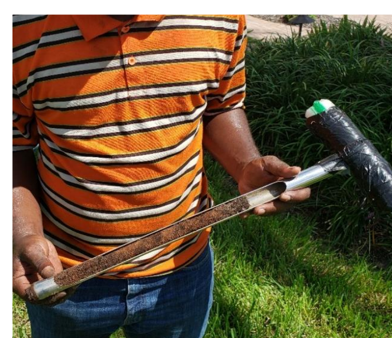
Figure 2. Punch tube used for soil sample collection.
